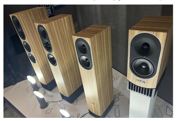
too high, where, of course, it will start to beam and get narrower, which is bad for making anything sound realistic. The wave guide also allows us to run the tweeter lower without having issues of power handling.
