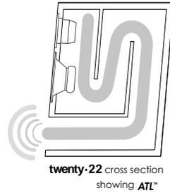
PMC's **ATL™** (Advanced Transmission Line) enclosures have taken loudspeaker design to the highest level.
