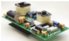
The EB1's 24dB/Oct hand built 31 element precision crossover
